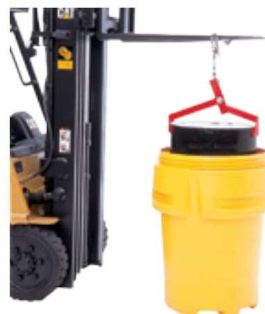
409 Drum Lifter - Securely grips 209L steel drums when loading and unloading salvage drums, Rugged, all-steel construction, Load capacity: 455 KG.
