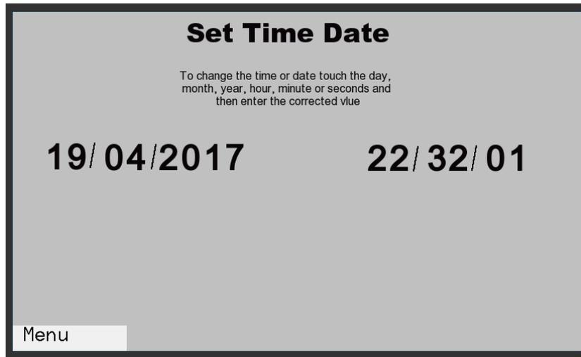
The time and date can be adjusted by tapping our touch screen either the time or the date and then entering the new or correct time and date. The system will hold the correct time or date for up to 2 years without power.
